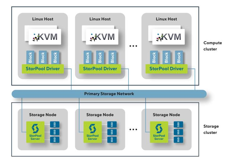
Disaggregated deployments use dedicated servers for the storage system and the compute cluster. This type of deployment is preferred when purpose-optimized hardware will bring more value than a reduced total number of nodes. This type of deployment simplifies the independent scaling of storage and compute resources. The
